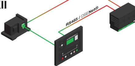
Connecting your DSE Intelligent Battery Charger to the DSE73XX MKII control module gives access to a wealth of useful battery charger information.
